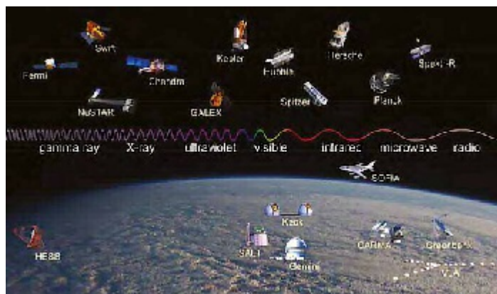
Figure 1: Sample of telescopes (operating as of February 2013) at wavelengths across the electromagnetic spectrum. (Source: NASA)
